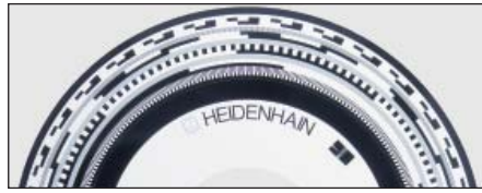
Conventional graduated disk with 13 Gray-code tracks
